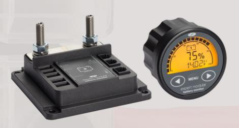
The Expert Modular can monitor up to three battery banks. The inputs for battery bank 2 and 3 can also be configured for other purposes, like mid-point voltage measurement, keyswitch input, setup lock or backlight control. The Expert Modular battery monitor can measure DC currents up to 600Amps (500Amp continuous) and voltages up to 70Vdc. So any lead- or lithium based battery from 12V up to 48V can be monitored.
