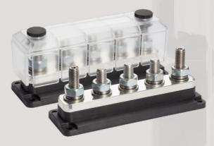
All DC Modular products are equipped with stainless steel studs, washers and nuts for optimal corrosion resistance. Tin plated high purity copper busses provide maximum conductivity, reducing heat and improving efficiency. The base material used for the DC Modular products is made from a special, fiber reinforced compound. This material offers excellent high temperature properties, good chemical resistance and high strength.
